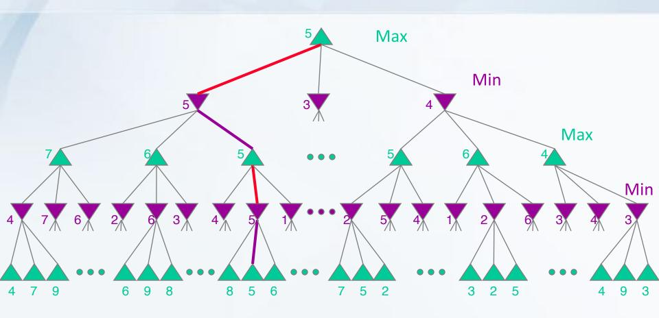
moves by Max and countermoves by Min
